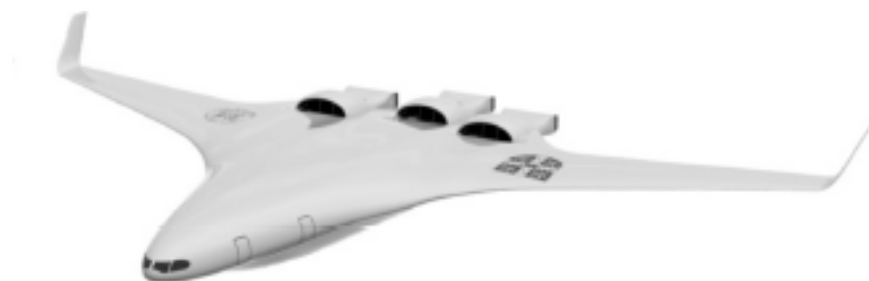
Figure 1.2 A concept of hybrid wing aircraft [11]
