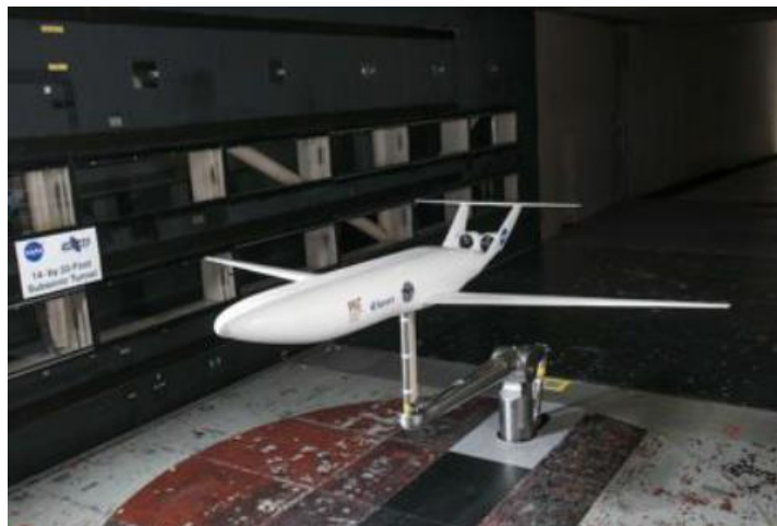
Figure 1.5 D8 transport aircraft concept [13]
