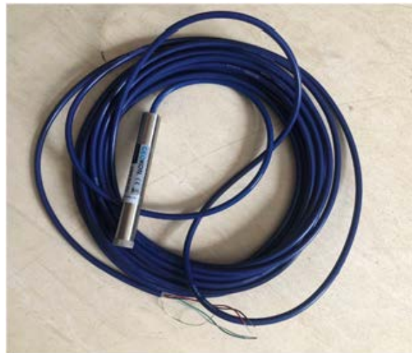
Figure A.11 Photo of the piezometer with a 0.14 m height
