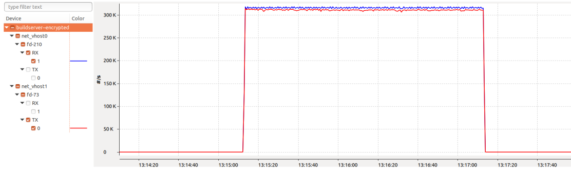
Figure 5.8 The rate of packet forwarding is lower than the rate of the packet reception.
