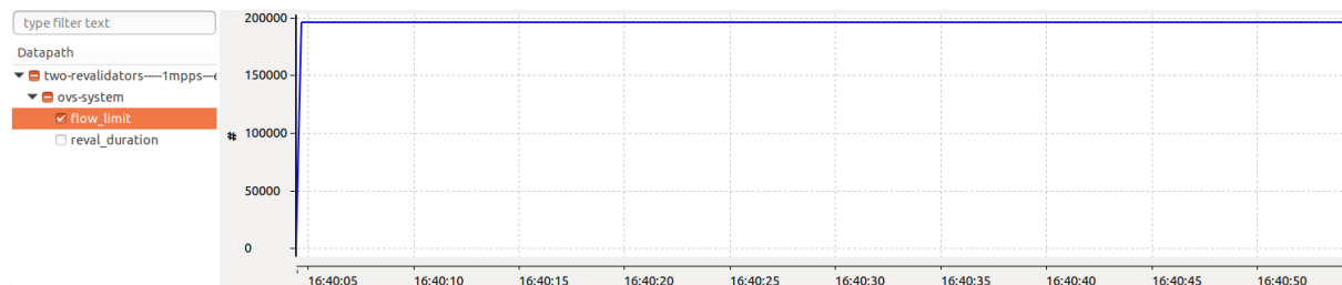
Figure 4.10 Variation of the flow-limit value after fixing the issue (adding another revalidator thread)
