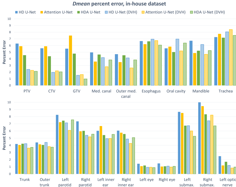
FIGURE 5.4 Dose mean percent error per structure for each model on the in-house dataset.
