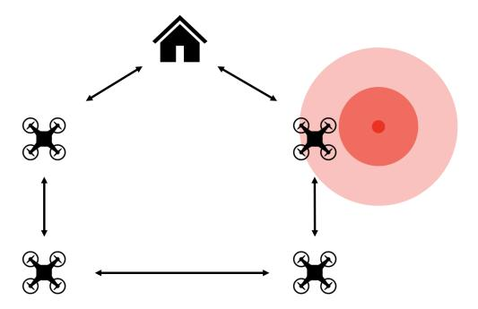
Figure 3.20 A simplified graph description of the physical testing environment. The decaying radiation source is represented by the concentric red circles. The base station, at the top of the figure, is also a drone.
