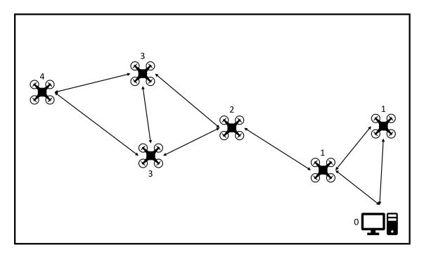
Figure 3.2 An example of minimal hop count towards the base station (bottom right) values held by robots after building the routing table.
