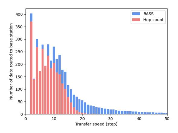
Figure 3.14 RASS transmission speed (random topology)
