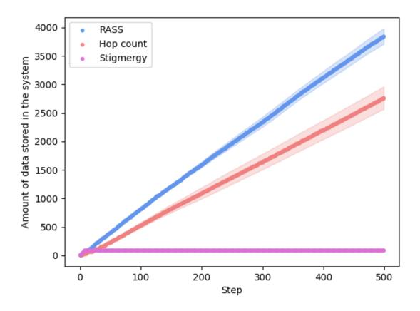
Figure 3.18 RASS storage capacity (random topology)
