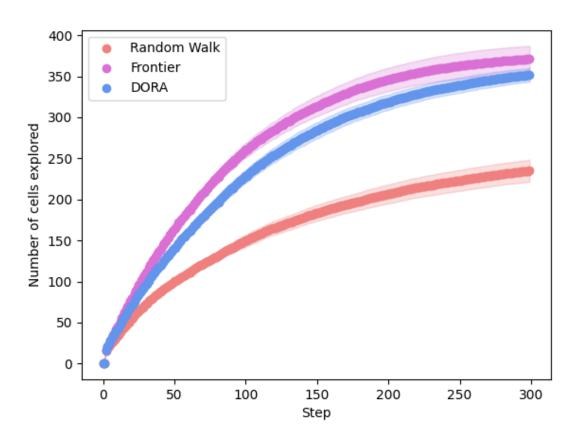
Figure 4.10 DORA cell exploration performance (N=20 robots)
