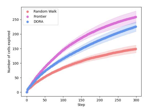
Figure 4.8 DORA cell exploration performance (N=10 robots)
