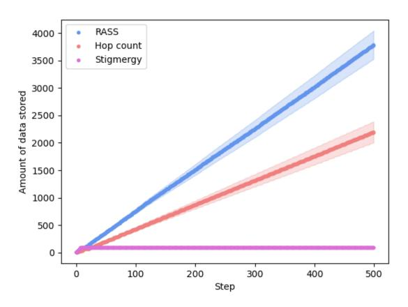
Figure 3.15 RASS storage capacity (grid topology)
