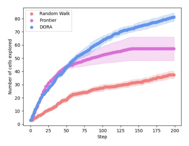
Figure 4.11 DORA cell exploration performance (N=5 physical robots)
