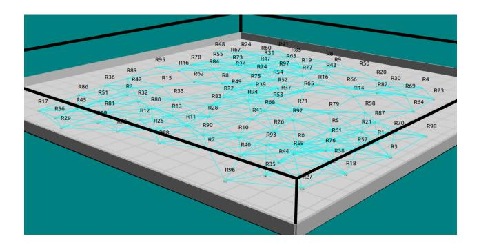
Figure  $3.5~400 \rm m^2$  environment in the ARGoS simulator with 100 KheperaIV robots in a formation obtained through Lennard-Jones potential interactions.
