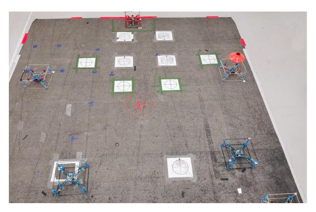
Figure 3.19 Physical disposition of the 3x3m environment with 5 drones and a radiation source (red cone).
