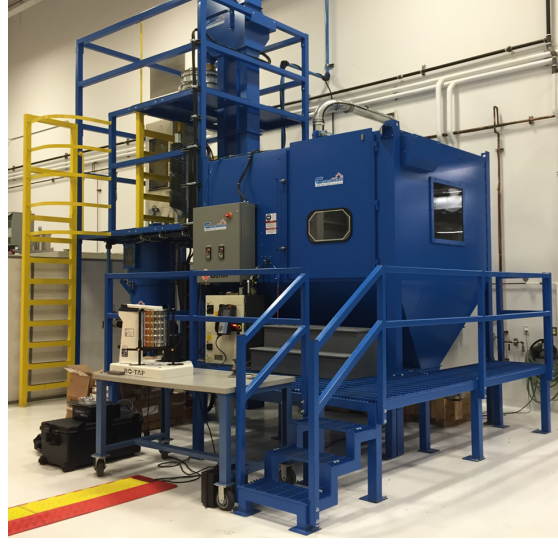
Figure 4.2 Shot peening machine consists of air-compressed peening cabinet for shot peening. The media are projected from a pressurized tank into the cabinet where they shot the parts.
