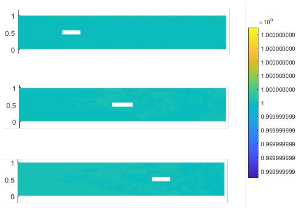
Figure 5.49 Pressure distributions on reference grid at initial position, mid-trajectory, and at the end of trajectory. The position of the hole changes with the mobile grid motion.
