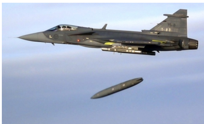
Figure 1.1 The Gripen E aircraft performing the separation test of the drop fuel tank [1].
