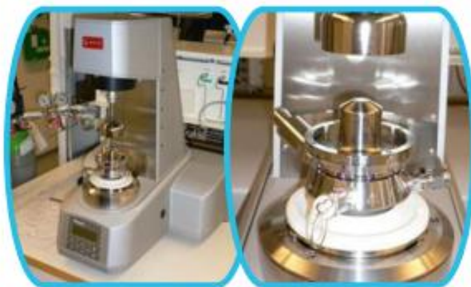
Figure 3.2– Apparatus (MCR 501 Rheometer from Anton Parr Canada)
