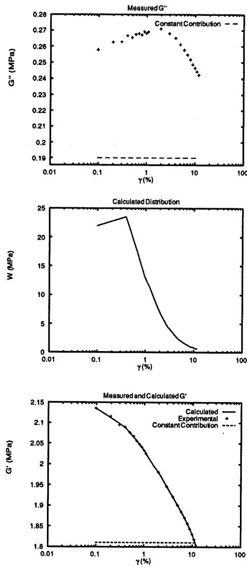
Figure 15: From top to bottom: experimental values of  $G''(\gamma)$  for SBR/N762 composite; computed values of  $W(\gamma_b)$  for SBR/N762 composite; computed and experimental values of  $G'(\gamma)$  for SBR/N762 composite.
