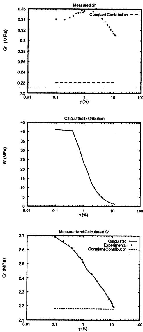
Figure 14: From top to bottom: experimental values of  $G''(\gamma)$  for SBR/N550 composite; computed values of  $W(\gamma_b)$  for SBR/N550 composite; computed and experimental values of  $G'(\gamma)$  for SBR/N550 composite.
