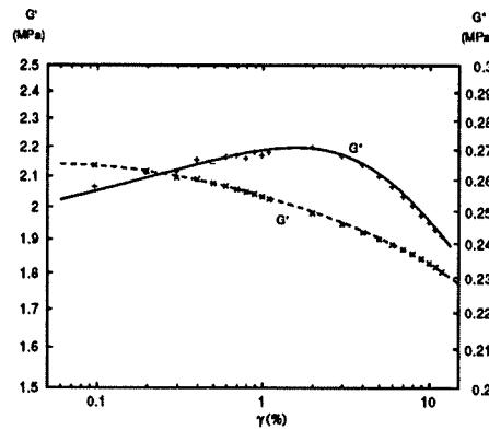
Figure 1: Typical relation between Coulomb modulus and amplitude of deformation
