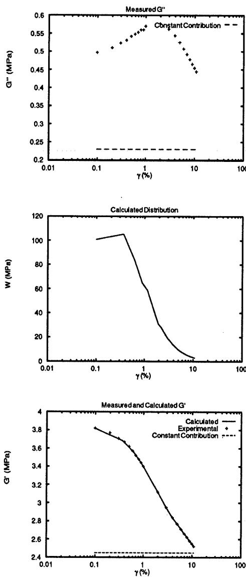
Figure 13: From top to bottom: experimental values of  $G''(\gamma)$  for SBR/N330 composite; computed values of  $W(\gamma_b)$  for SBR/N330 composite; computed and experimental values of  $G'(\gamma)$  for SBR/N330 composite.
