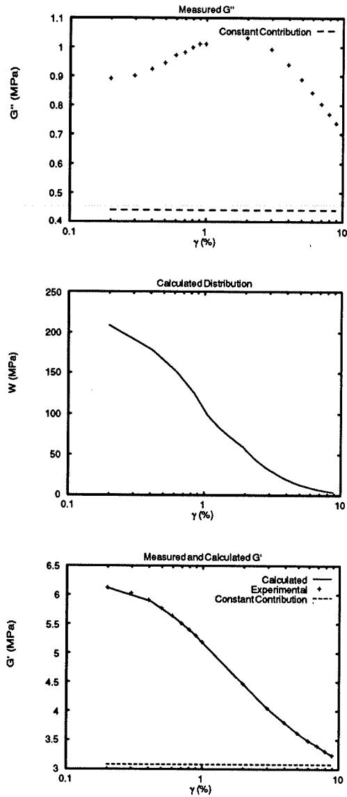
Figure 12: From top to bottom: experimental values of  $G''(\gamma)$  for SBR/N110 composite; Computed values of  $W(\gamma_b)$  for SBR/N110 composite; Computed and experimental values of  $G'(\gamma)$  for SBR/N110 composite.
