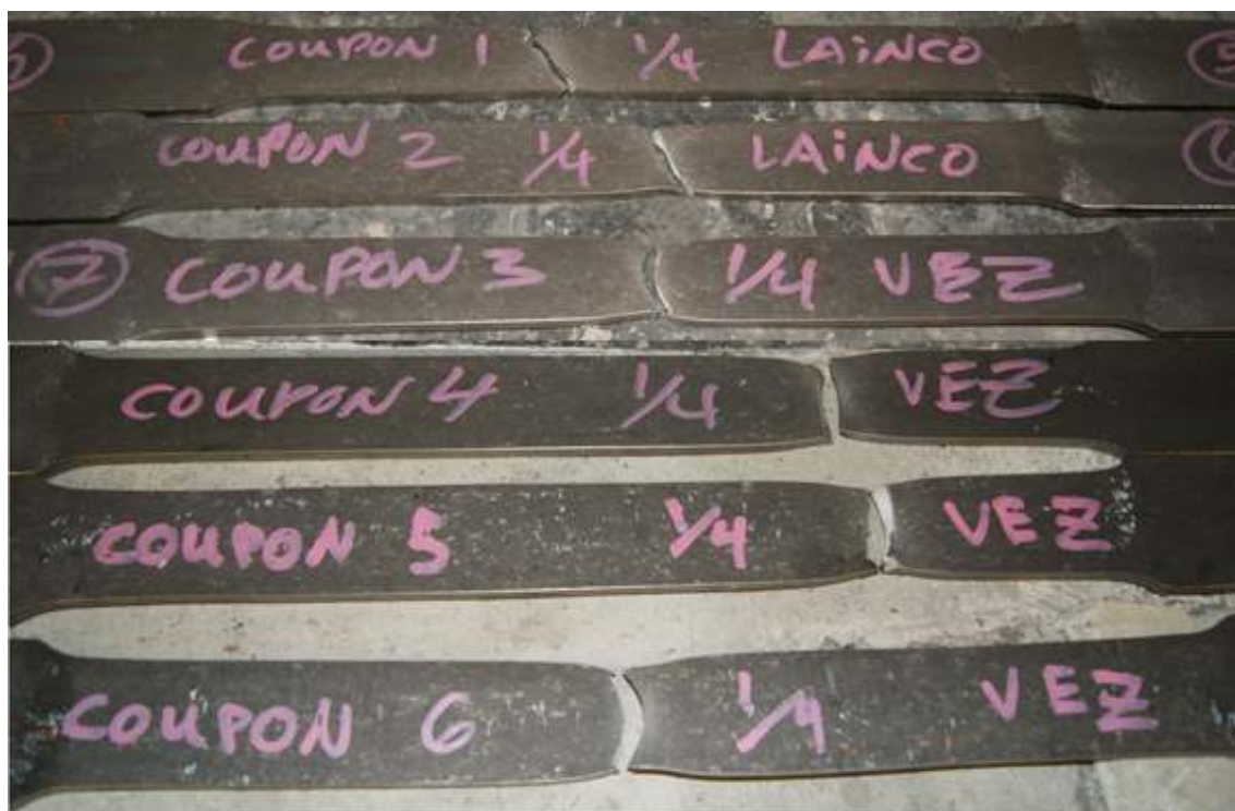
Figure 3.21: Rupture des six coupons, C-B-P250
