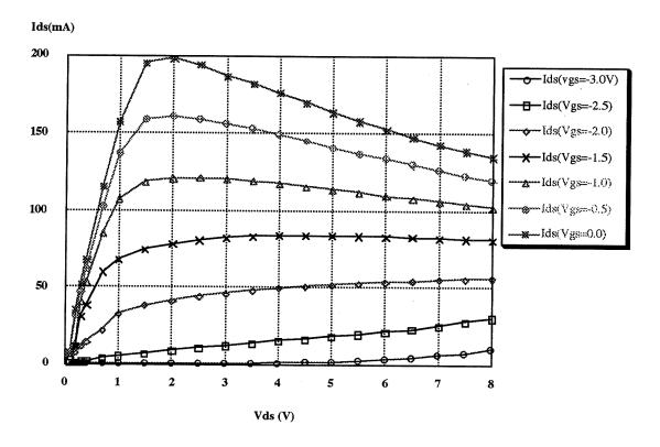
Fig. 2. DC characteristics of the MESFET
