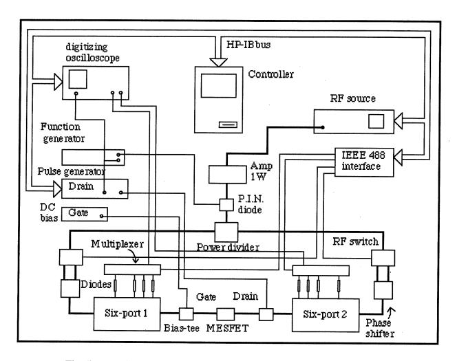
Fig. 5. Experimental setup used for the S-parameter measurements.
