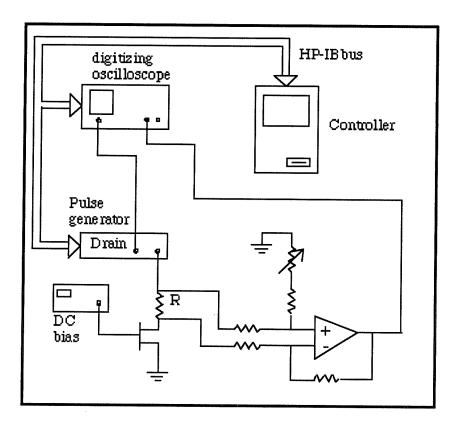
Fig. 3. Pulsed I-V measurement setup.
