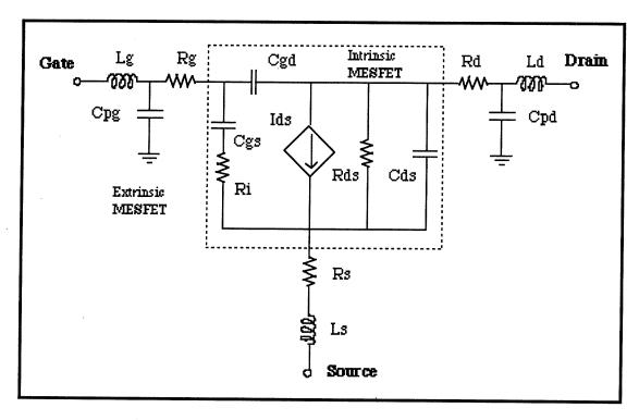
Fig. 1. Small-signal equivalent circuit of the MESFET.
