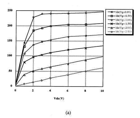
Fig. 4. Ids versus Vds (a) after  $24\mu s$  (b) after 1.4s from the beginning of the pulse.
