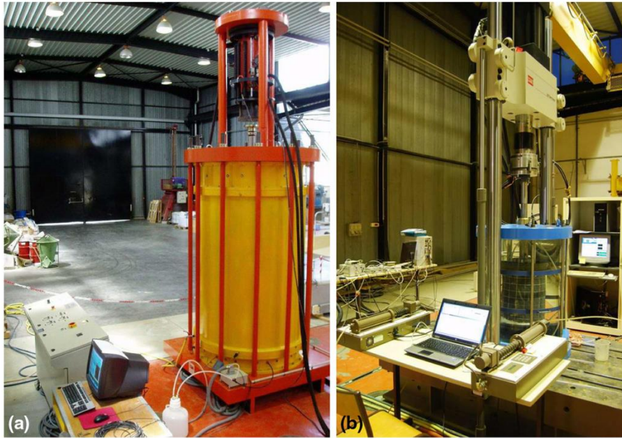
Figure 2.6: Large-scale triaxial test apparatus; (a) 1000 mm diameter and (b) 250 mm diameter (Ovalle et al. 2014). The tested materials were rock aggregates with maximum particle size 40 mm and 160 mm and uniformity coefficient 2.
