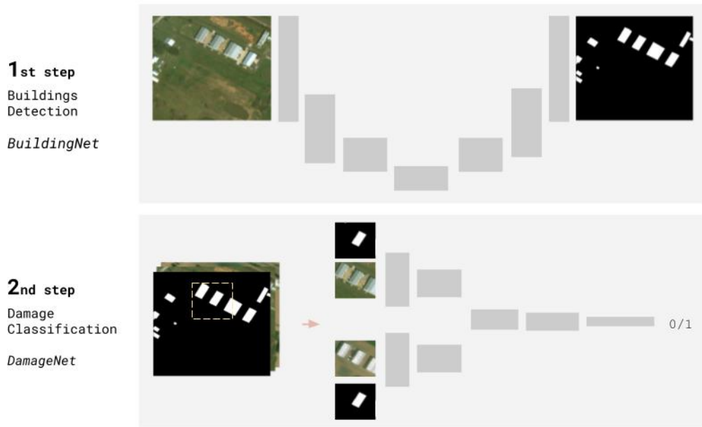
Figure 3.8 Two-step modelling approach composed of (1) a Building Detection model ( BuildingNet ) and a (2) Damage Classification model ( DamageNet ). The input of BuildingNet is a pre-disaster image, the output a binary segmentation heatmap, i.e. that each pixel has a sigmoid output. The input of DamageNet is both the pre- and post-disaster image patches centred on a single building along with the building mask. The two models are applied sequentially.
