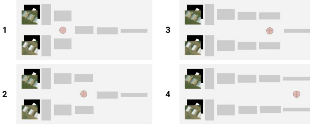
Figure 3.11 Ablation study configurations for the fusion of the pre- and post-disaster streams after the first (1), second (2), third (3) and fourth (4) blocks.
