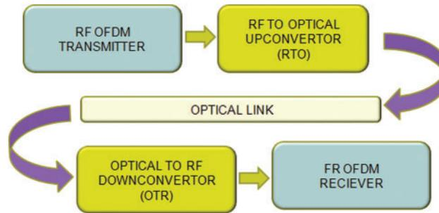
**Figure 1:** Block diagram of a generic CO-OFDM system
