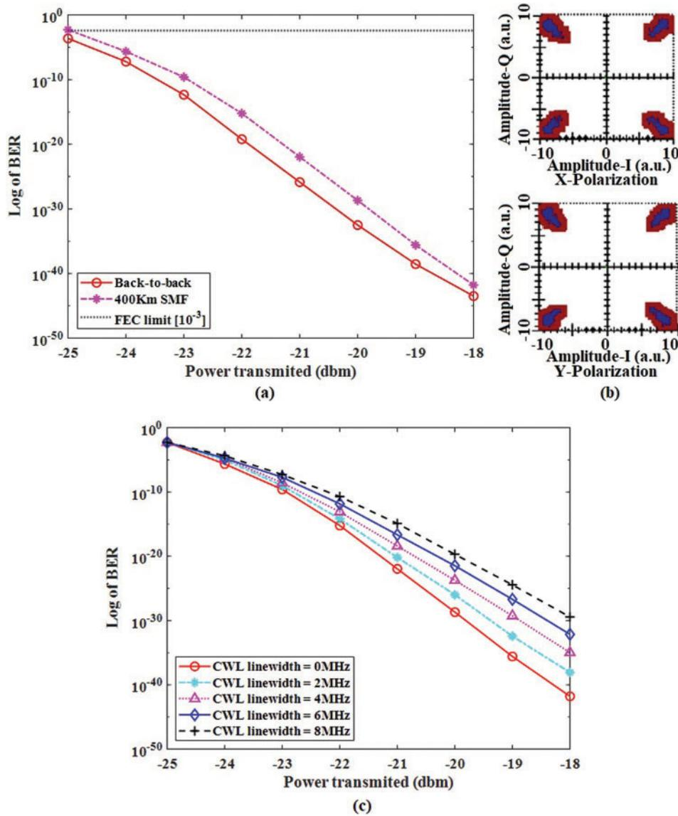
**Figure 4:** (a) BER as a function of launched power into the transmitter for 400 km SMF transmission (b) X- and Y-polarization constellation diagrams (c) variation in BER vs. the launched power with CW laser linewidth variation
