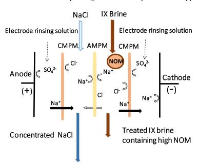
Figure 1. A schematic illustration of the MSED stack used for the IX spent brine desalination.
