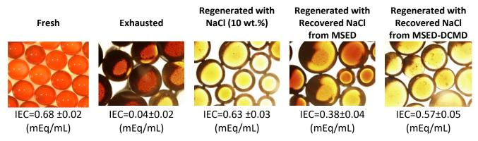
**Figure 7.** Microscopic images of the fresh, exhausted and regenerated IX resins used in the NOM removal process (scale: 500 μm). (The image of the fresh resins was provided by its supplier).
