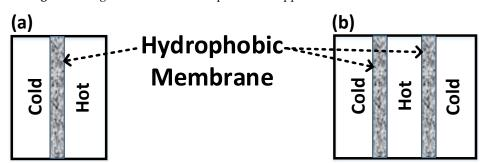
Figure 3. DCMD (a) conventional and (b) modified stack configurations.
