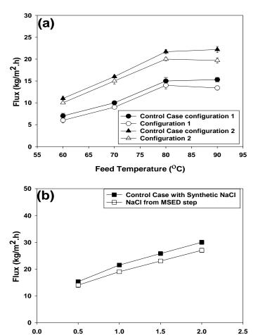
Figure 6. Transmembrane flux as a function of (a) feed temperature, (b) feed flow rate.
