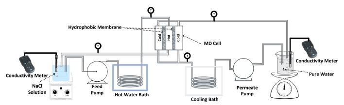
Figure 2. Diagram of the DCMD experimental apparatus.
