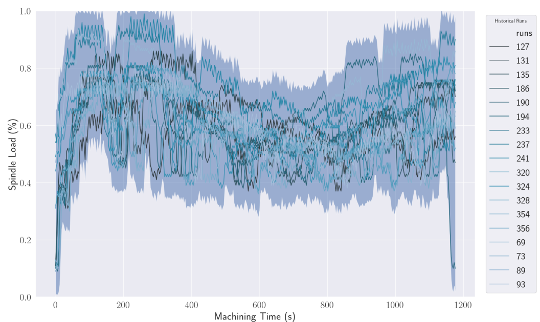
Figure 7. Program 1543 tool 6040 on machine T5-1 normal behavior extraction.
