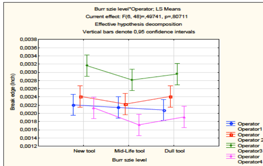
Figure 6-20 : Effect of burr size and operator on break edge (Part B)
