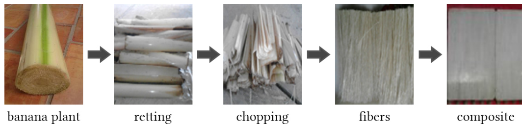
Figure 1. Extraction of fibers from the banana plant and the final composite laminate.
