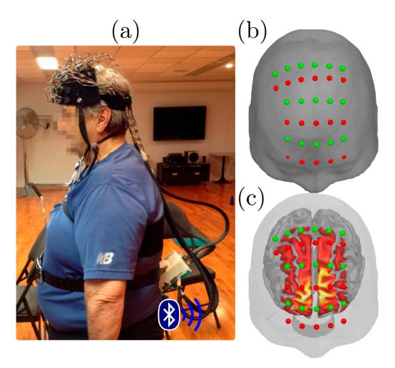
**Figure 1.** Functional Near-Infrared Spectroscopy (fNIRS) experimental setup. (a) Participant wearing the NIRS device consisting of a frontal cap wired to a Bluetooth acquisition device (b) Frontal view of the optode layout with sources in red and detectors in green, overlaid on the Colin27 anatomical template. (c): cortical sensitivity map for the fNIRS measurements covering the central part of the prefrontal cortex, overlayed with fNIRS montage and the scalp surface.
