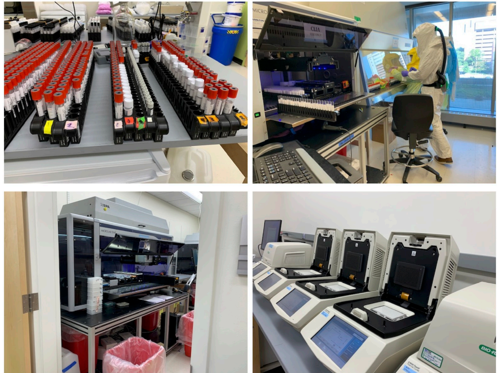
Fig 3. Laboratory process steps. (Top left) Samples racked and scanned; note the many different sizes and shapes. (Top right) Tubes are uncapped and deswabbed manually then placed on the deck of the Hamilton STARlet for transfer to deep-well plates. (Bottom left) Deep-well plates stacked in front of a Hamilton STAR for RNA extraction. (Bottom right) qPCR in progress and completed.
