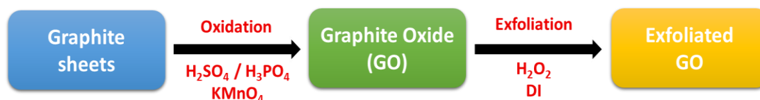
Figure 6-1 A scheme of GO preparation
