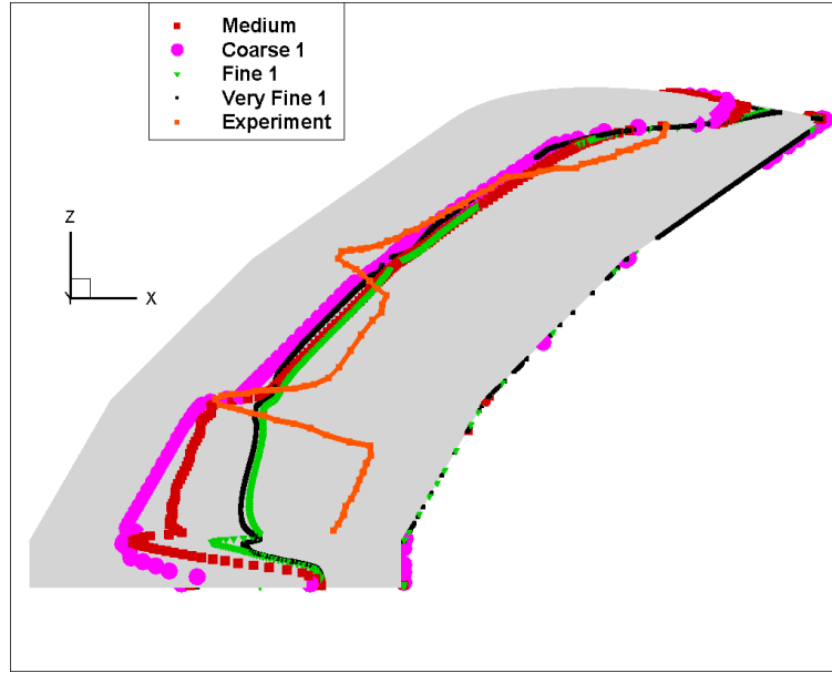
Figure 5.6 Transition lines along the Sickie-shaped wing for several grid refinements and varying wall spacing ( M = 0.16 , Re = 2.75 * 10^6 , FSTI = 0.0017 , \mu_t/\mu_l = 10 , \alpha = -2.6^\circ )
