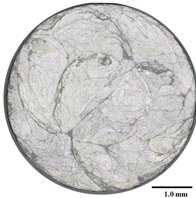
Figure 6.10 Cross-section image of the carbon fiber/PEI braid-truded rod.
