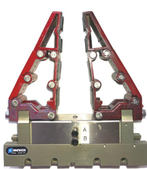
Figure 4.1 PaCoMe fingers prototype on a Schunk gripper.
