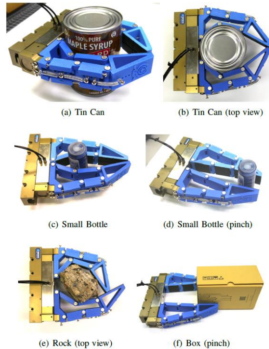
Figure 2.6 Grip tests performed by the PaCoMe finger, taken from (Birglen, 2015)
