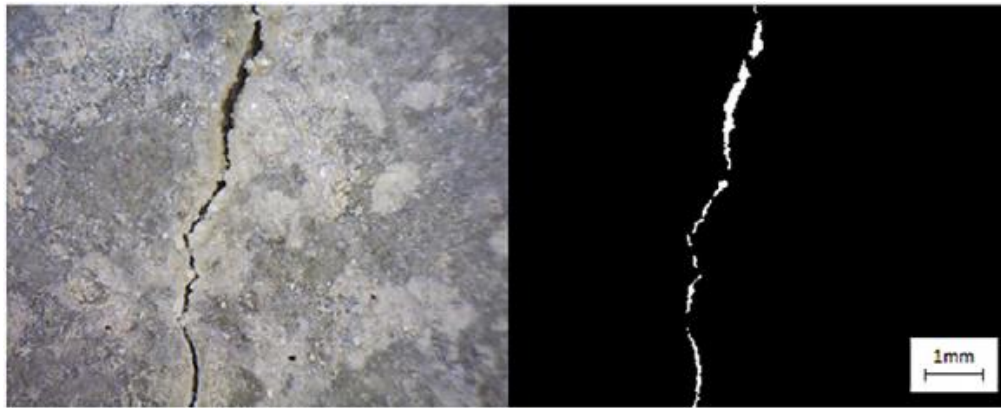
Figure 2.9. Example of binary image of the crack (Cuenca et al., 2018)
