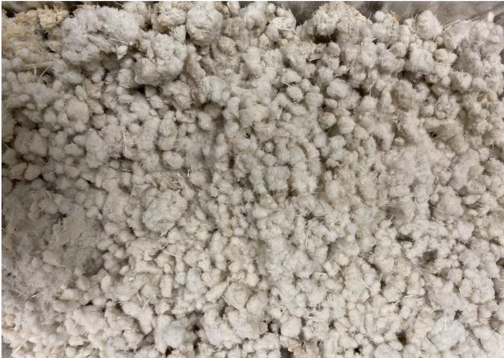
Figure 3.1 wind turbine blades after grinding
