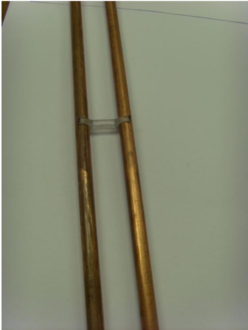
a) U-tube with spacer.
