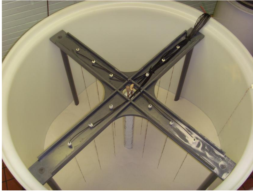
a) String rack in the partially-filled sand tank.
