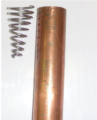
a) Conical spring machined for the mixing section.
