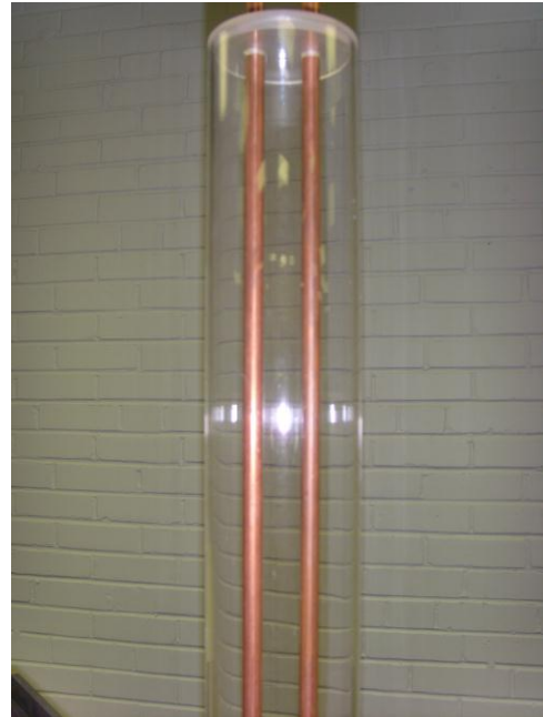
b) Top cap of the borehole which positions the U-tubes properly.
