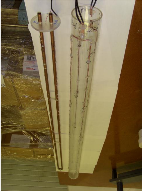
a) Borehole with surface thermocouples, ready to be filled with glass beads.
