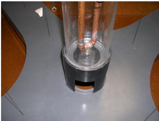
c) Seat of the borehole and the bottom cap on which the U-tube is centered from bottom.
