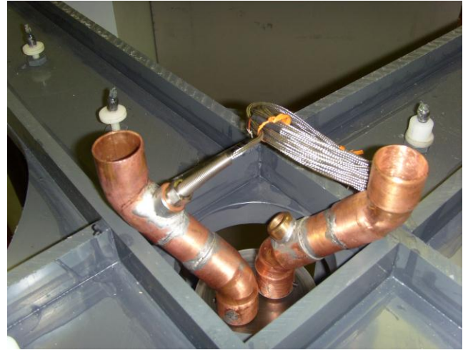
b) Outlet (left) and inlet (right) thermistors and their fittings.
