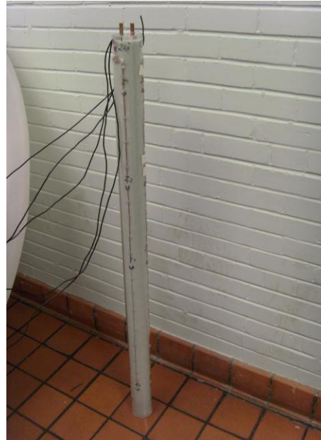
b) Borehole filled with glass beads, ready to be installed on the string rack.
