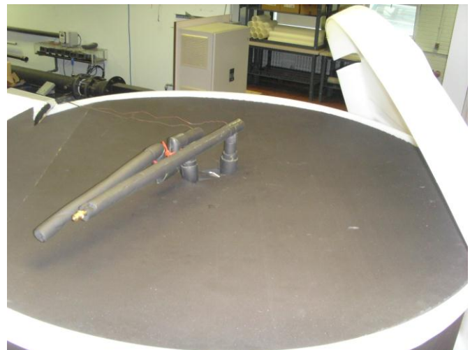
d) Insulated inlet and outlet temperature fluid measurement sections.
