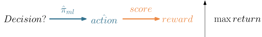
Figure 5.6 When learning through a reward signal, no expert is involved; only maximizing the expected sum of future rewards (the return) matters.
