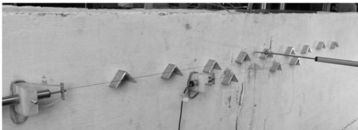
Figure 5-33: Barrier Longitudinal Deformation Sensors
