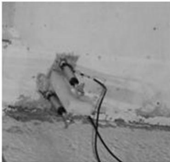
Appendix B Figure 4: Barrier and Injected Mortar Separation
