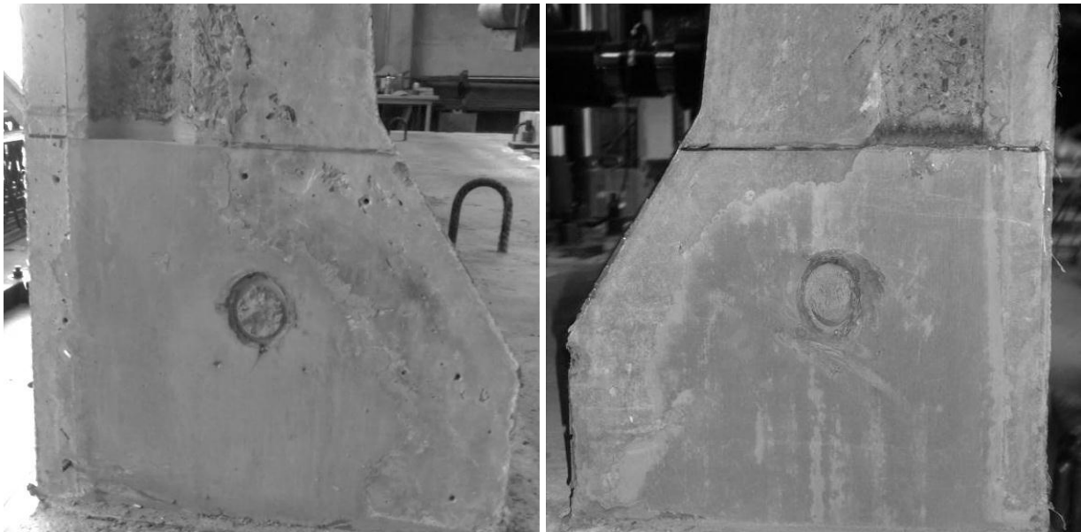
Figure 5-29: Ends of Hollow Recess after Injection
