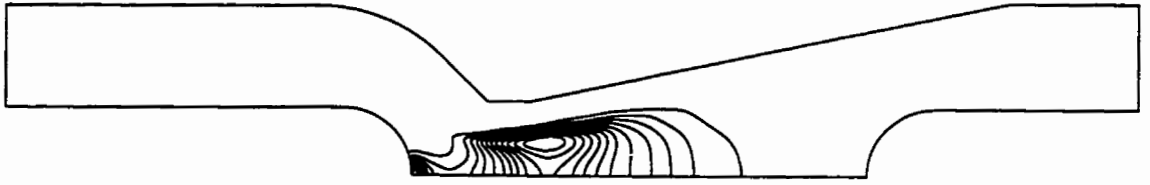
Figure 5.55: Rayonnement incident dans la bande 1: (min; max) = (-6,673 \times 10^1; 7,227 \times 10^4) \text{ W/m}^2
