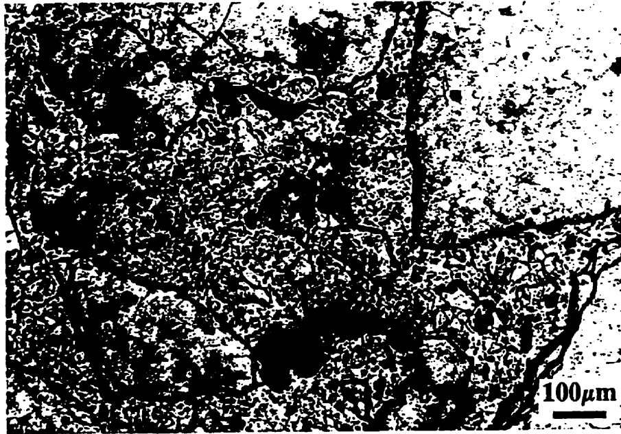
Figure 4.10 Microstructure of Magnesia Based Castable (F2) After firing at 1600°C
