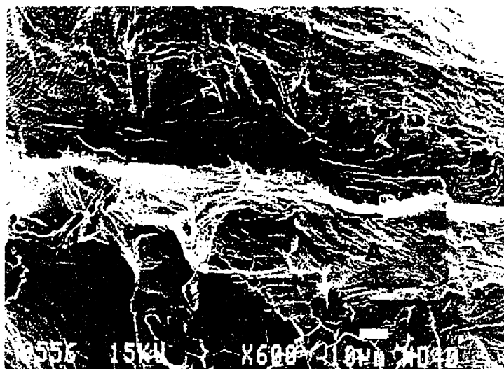
Figure 3.17 Transgranular fractured \delta -ferrite (F) is separated by a transition stretch zone in austenite (A) in the hydrogen-induced cracking zone, in the same specimen as Fig. 3.15.
