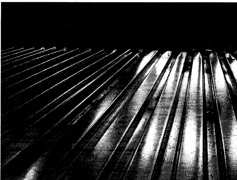
Figure 5.52 Buckling in top sheet preventing failure of weld to frame, Test 23
