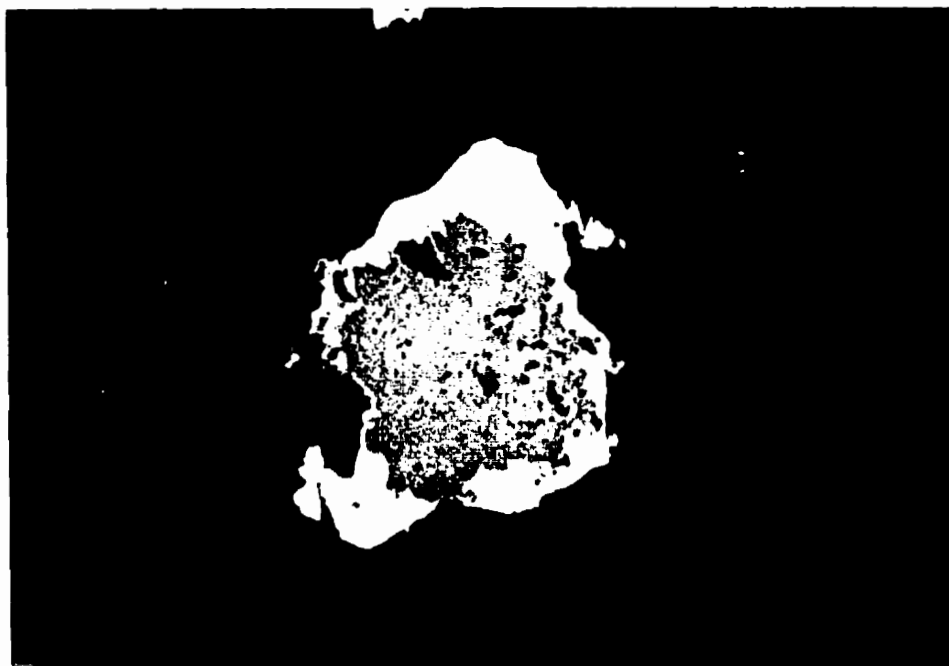
Figure 5.15: Purple bornite replaced by chalcocite. Note the presence of some chalcopyrite with the bornite. Sample 92, PTS, RL, FOV= 1 millimetre.
