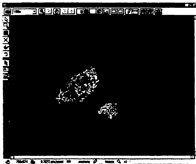
Figure 5.8: Modified image after the OR instruction was applied to bitplanes 1 and 8.
