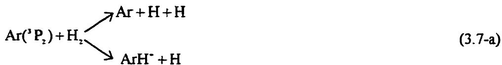
with k<sub>a</sub> = 6.6 × 10<sup>-11</sup> cm<sup>3</sup> s<sup>-1</sup> [23], following which the H atoms are excited by electron collision. Moreover, the Lyman α radiation is enhanced by the following energy transfer mechanism:
