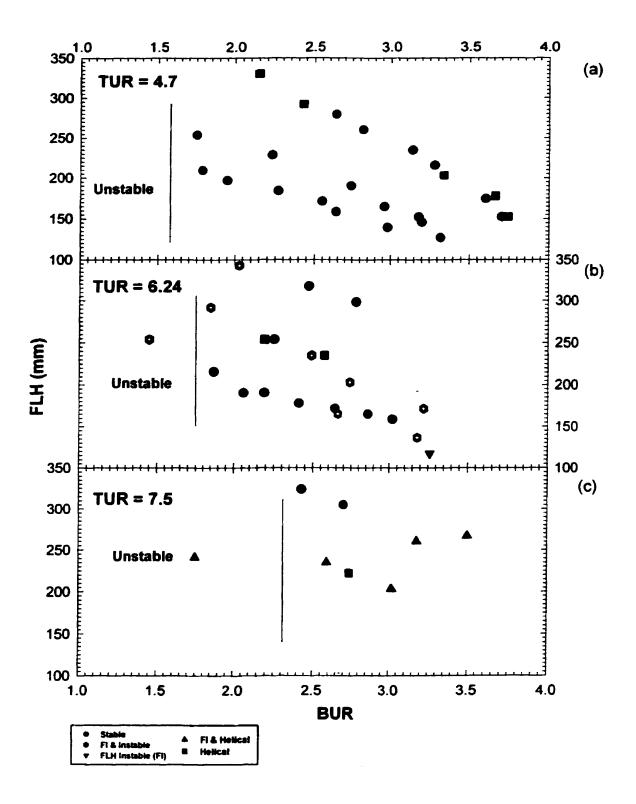
Figure 4.18. Bubble stability behavior of mPE under the extrusion temperature =  $200^{\circ}$ C, Flow rate = 5.4 Kg/h (a) TUR = 4.7, (b) TUR = 6.24, (c) TUR = 7.5.
