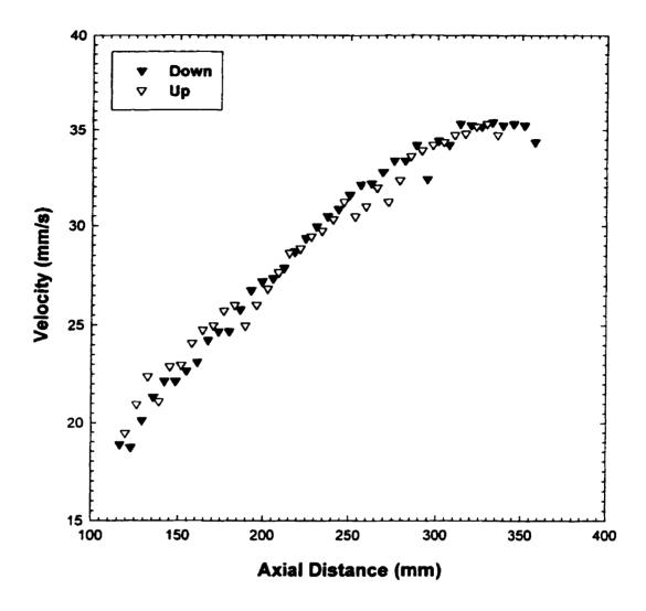
Figure 4. 11. Bubble velocity profiles along the length for LDPE. Polymer flow rate = 5.91 kg/h, extrusion temperature = 2000C, BUR =  $1.73 \cdot \text{FLH} \approx 300 \text{mm} \cdot \text{TUR} = 3.80$
