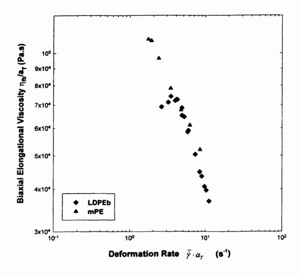
Figure 4.23. Biaxial elongational viscosity versus deformation rate at the reference temperature of 170°C for LDPEb and mPE during film blowing. The film blowing conditions are the same as in Figure 4.10.
