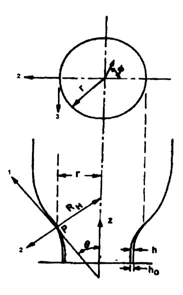
Figure 3. 5. Local rectangular Cartesian coordinate system describing the deformation of a bubble (adopted from Han and Park, 1975).
