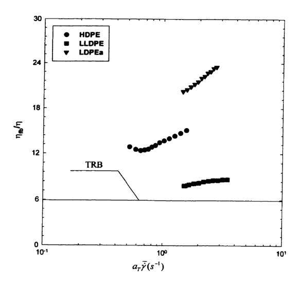
Figure 4.25a.  $\eta_{fb}/\eta$  versus  $a_T \bar{\gamma}$  at the reference temperature of 170°C for HDPE, LLDPE and LDPEa during the film blowing. The film blowing conditions are the same as in Figure 4.24.
