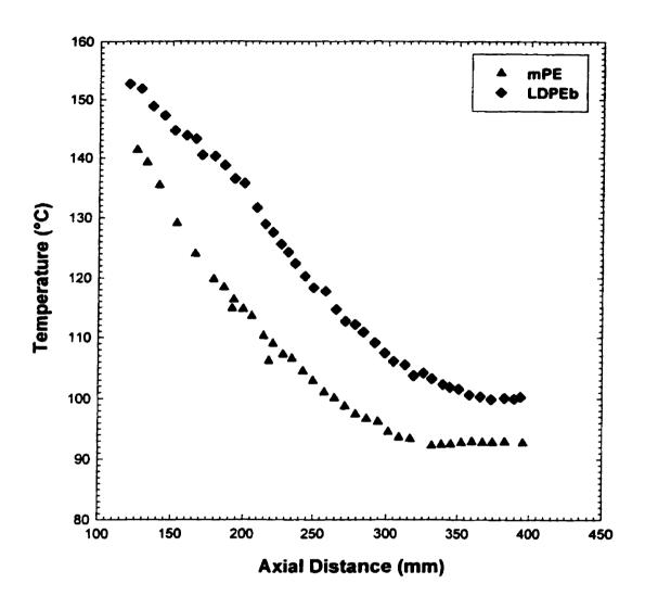
Figure 4. 10. Bubble Temperature along the axial distance for mPE and LDPEb. The Mass Flow Rate = 6.5 Kg/h, TUR = 6.0, BUR = 2.5, Temperature = 200 °C, FLH  $\approx 300mm$
