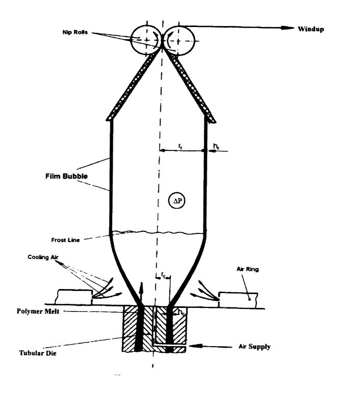
Figure 1.1. Schematic Diagram of the film blowing process.
