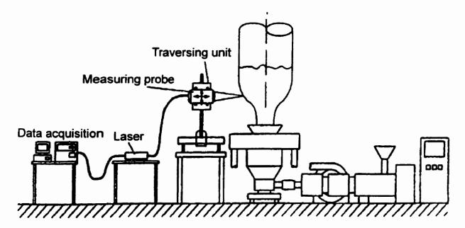
Figure 3. 4. Experimental setup on LDV measurement.
