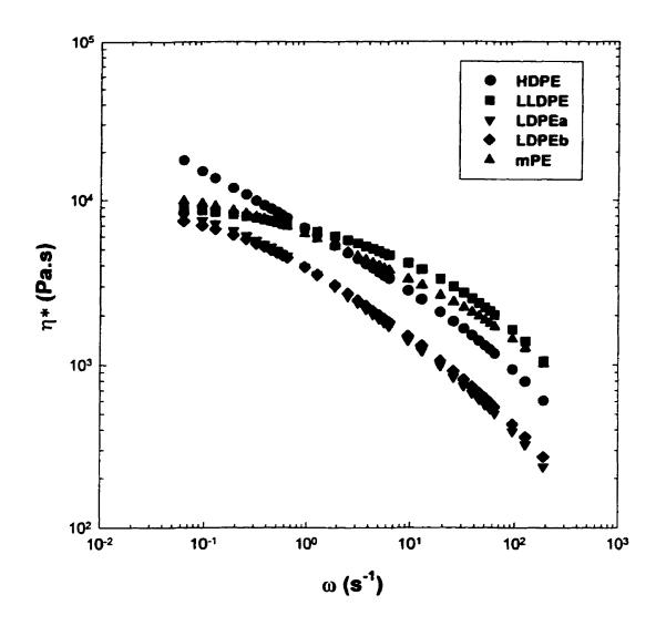
Figure 4. 1. Complex viscosity data versus frequency for five resins at 200°C.
