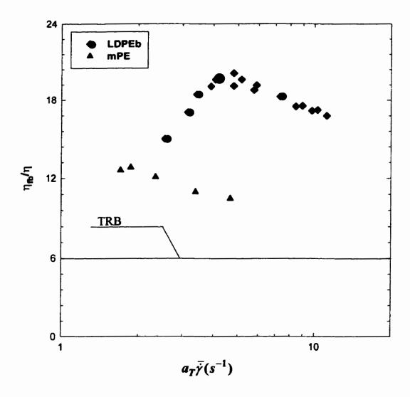
Figure 4.25b.  $\eta_{be}/\eta$  versus  $a_T \bar{\gamma}$  at the reference temperature of 170°C for LDPEa and mPE during the film blowing. The film blowing conditions are the same as in Figure 4.10.
