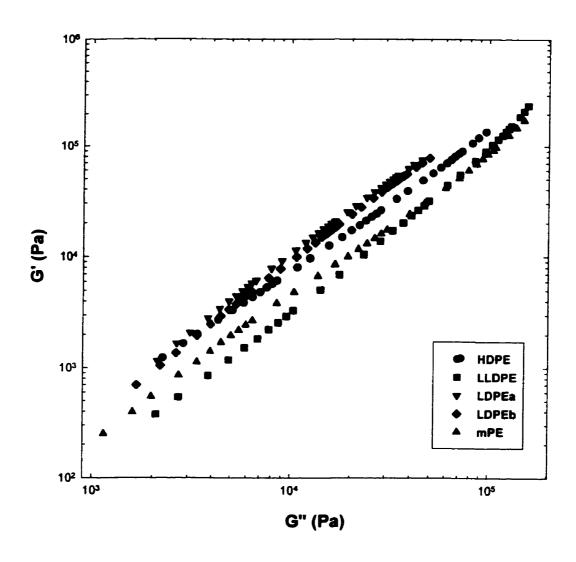
Figure 4.21. The comparison of  $\log G'$  versus  $\log G''$  for HDPE, LLDPE, LDPEa, LDPEb, and mPE.
