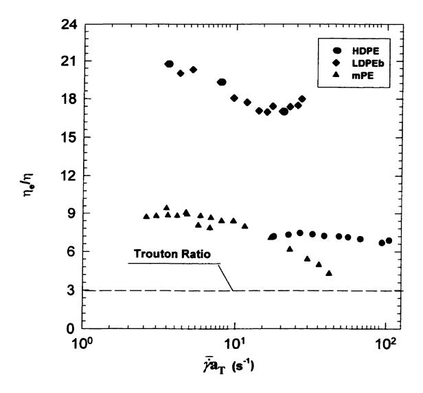
Figure 4. 9. Trouton Ratio for HDPE, LDPEb and mPE resins at the reference temperature as 170°C.
