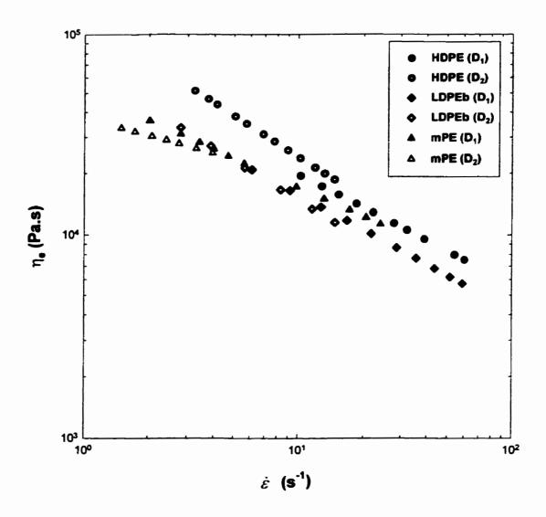
Figure 4.22. Comparison of elongational viscosity of HDPE, LDPEb, and mPE by using Binding analysis at the temperature of 200°C.
