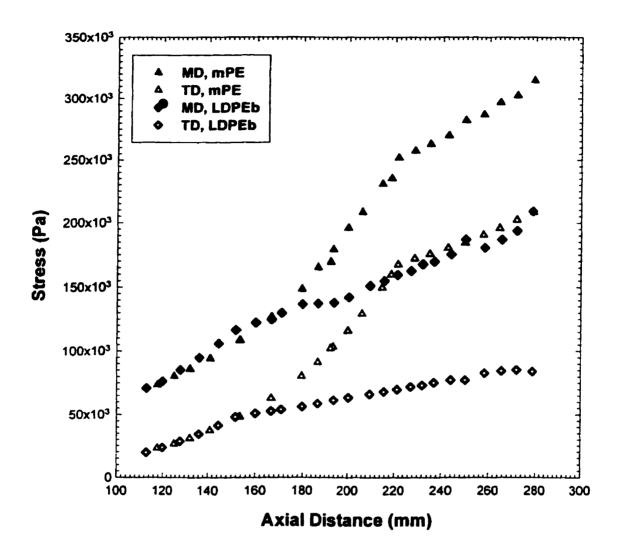
Figure 4.16. Stress profiles along the axial distance for mPE and LDPEb. The film blowing conditions are the same as in Figure 4.10.
