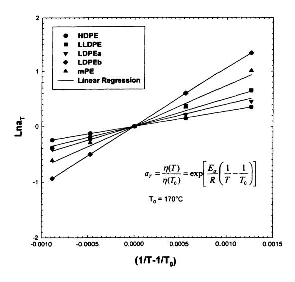
Figure 4. 6. Temperature shift factors by using Arrhenius equation at a reference temperature of 170°C.
