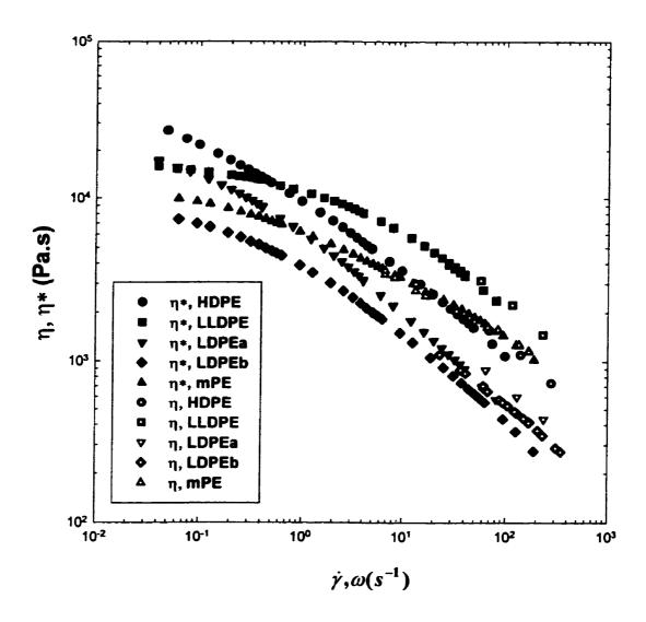
Figure 4. 7. Complex and steady shear viscosity data for five resins at 200°C.
