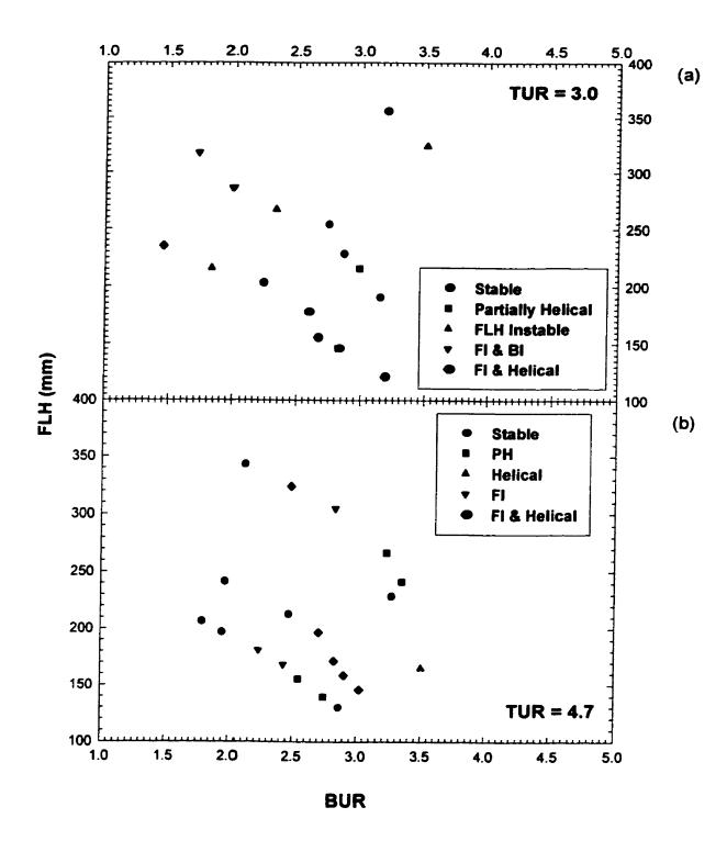
Figure 4.19. Bubble stability behavior of LLDPE under the temperature =  $200^{\circ}$ C, Flow rate = 5.4 Kg/h at (a) TUR = 3.0, (b) TUR = 4.7.
