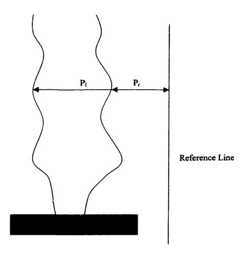
Figure 3. 7. Bubble instability measurement (adopted from Ghaneh-Fard et al., 1996b).
