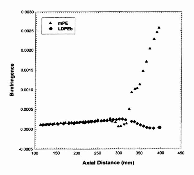
Figure 4. 15. Birefringence along the axial distance for mPE and LDPEb. The film blowing conditions are the same as in Figure 4.10.
