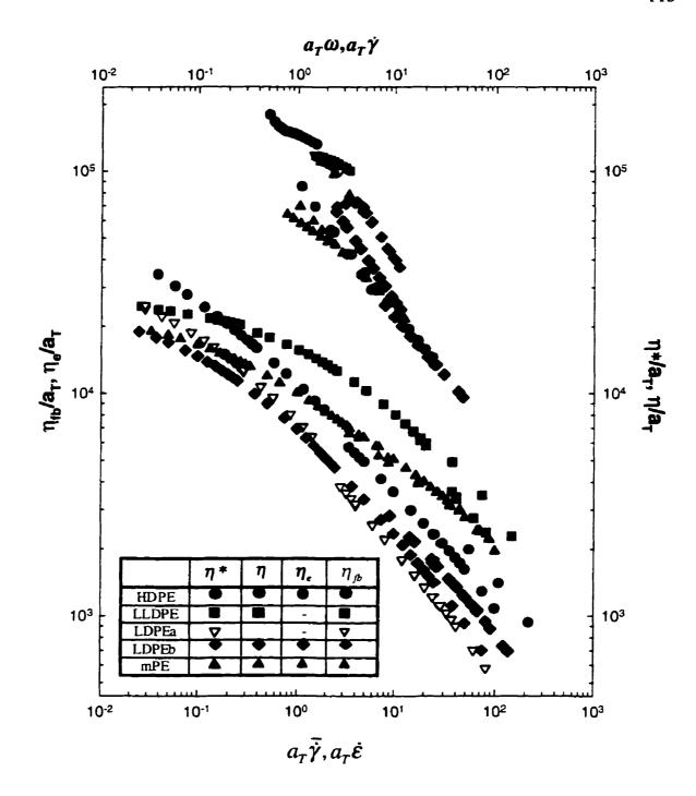
Figure 4.27. Complex, shear, uniaxial elongational, biaxial elongational viscosities versus frequency, shear rate, elongational rate, deformation rate respectively under the same reference temperature of 170°C for five resins.
