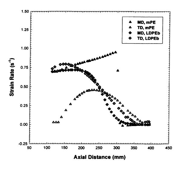
Figure 4. 14. Strain rates in MD and TD along the axial distance for mPE and LDPEb.
