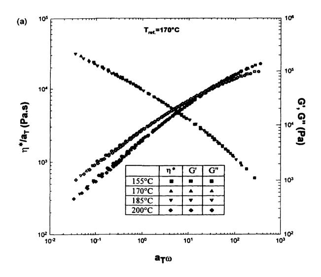
Figure 4. 5. Master curves for  $\eta^*$ , G', and G" at the reference temperature of 170°C for: (a) HDPE, (b) LLDPE, (c) LDPEa, (d) LDPEb, (e) mPE.
