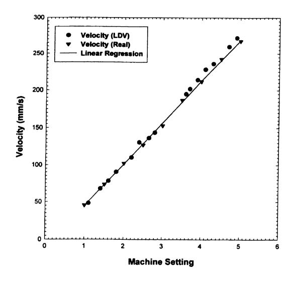
Figure 4. 12. Calibration of LVD.
