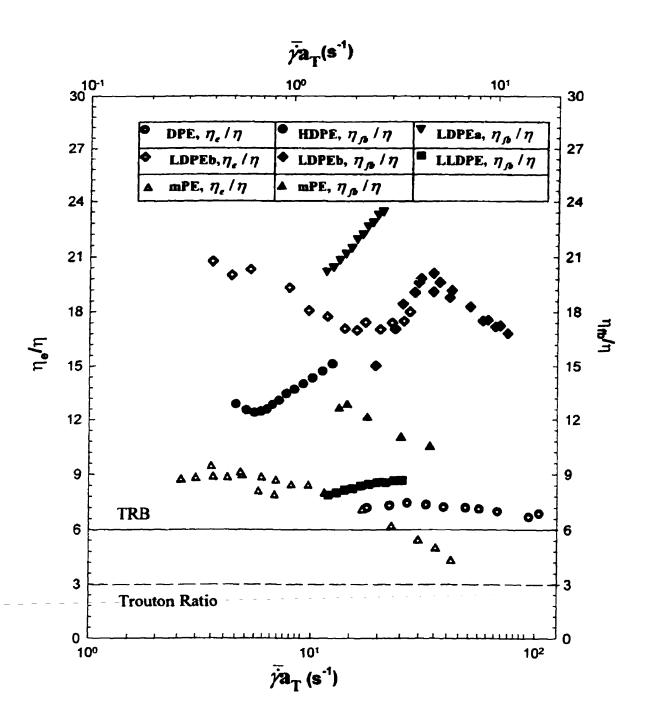
Figure 4.26. Comparison of Trouton ratio and TRB for five polyethylenes at a reference temperature 170°C.
