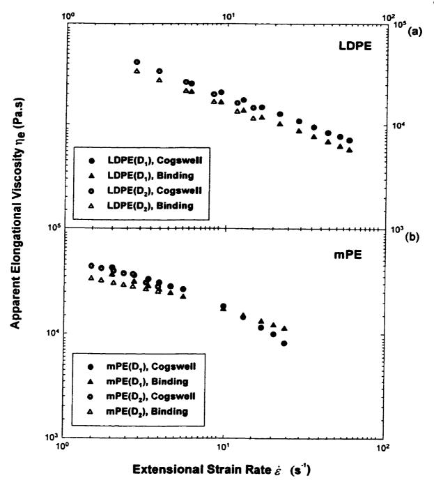
Figure 4. 8. Uniaxial Elongational Viscosity versus extensional rate for (a) LDPE and (b) mPE (c) HDPE at 200°C.
