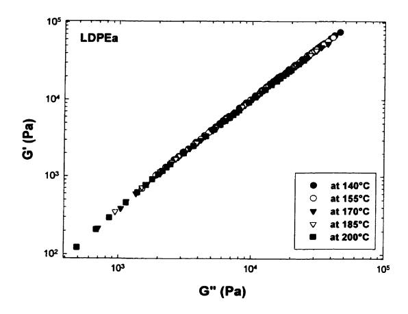
Figure 4.20.  $\log G'$  versus  $\log G''$  for LDPEa at five different temperatures.
