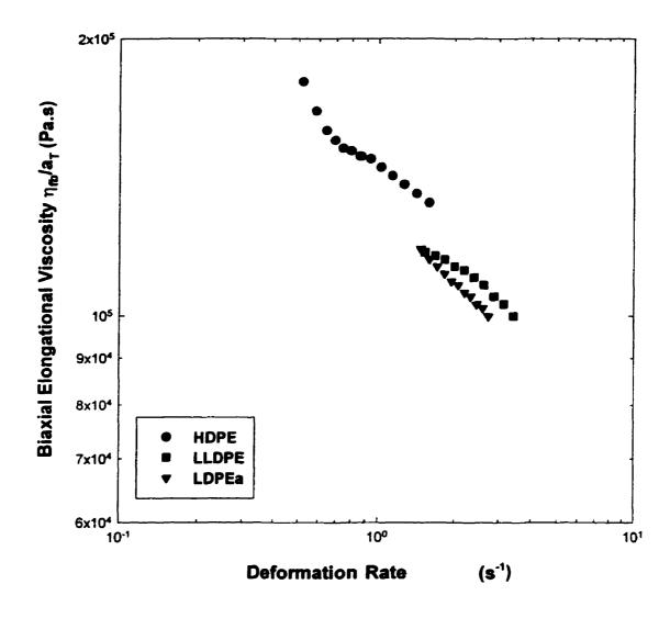
Figure 4.24. Biaxial elongational viscosity versus deformation rate at the reference temperature of 170°C for HDPE, LLDPE and LDPEa during film blowing. The flow rate = 4.05 kg/h, extrusion temperature = 220°C, TUR = 9.5. BUR = 2.0, FLH ≈ 250 mm (Calculated from experimental data of Ghaneh-Fard et al. 1997b)
