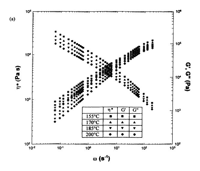
Figure 4. 4.  $\eta^{\bullet}$ , G', and G" versus  $\omega$  at five different temperatures for: (a) HDPE, (b) LLDPE, (c) LDPEa, (d) LDPEb, (e) mPE.
