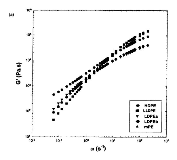
Figure 4. 2. The data of dynamic storage (a) and loss (b) moduli versus frequency for five resins at 200°C.
