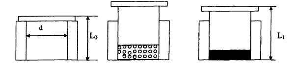
Figure 3. 2. Schematic diagram of measuring the density of molten polymer.
