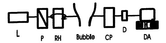
Figure 3. 6. Optical train for birefringence measurement. L-Light source, P-Polarizer, RH-Rotating half-wave plate, CP-circular polarizer, D-Detector, DA-Data acquisition (adopted from Ghaneh-Fard et al., 1996a)
