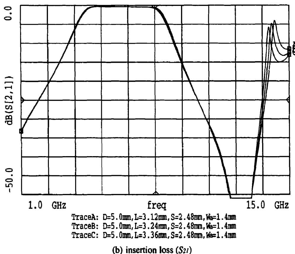
Figure 4.13 Simulated frequency response of the bandpass filter using the HP Momentum software: Group (II)
