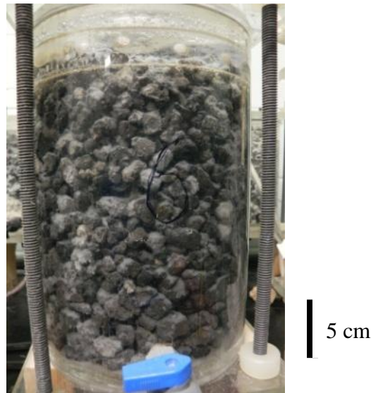
Figure 2.5 : Example of a 3-liter column filled with slag.
