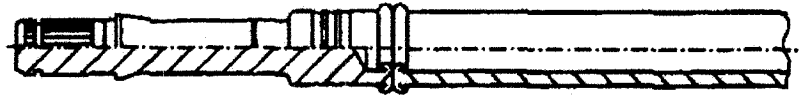
Figure 1.3: Bar shaft drilled and friction-welded. P. Amborn, H. Frielingsdorf, S.K. Ghosh and K. Greulich (1995) [2]
