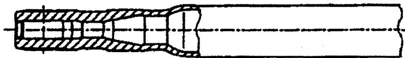
Figure 1.6: Monobloc tube shaft, outside contour stepped with different wall thickness. P. Amborn, H. Frielingsdorf, S.K. Ghosh and K. Greulich (1995) [2]
