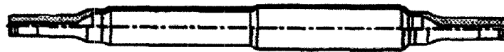
Figure 1.16: Hydraulic expansion formed tube shaft with swaged ends. P. Amborn, S.K. Ghosh and I.K. Leadbetter (1997) [3]
