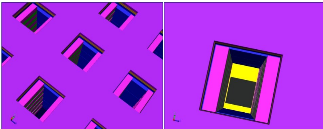
Fig 3.3: 3D schematic view of the microelectrode array
