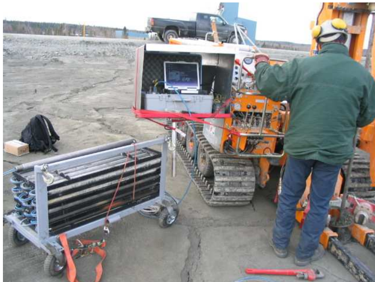
Figure 3-4 - Operation of the CPT rig.
