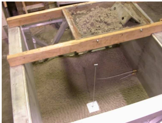
Figure 2-24 – Preparation of a sample for shaking table testing by air pluviation with tamping (Photo by Darcy Joliette).
