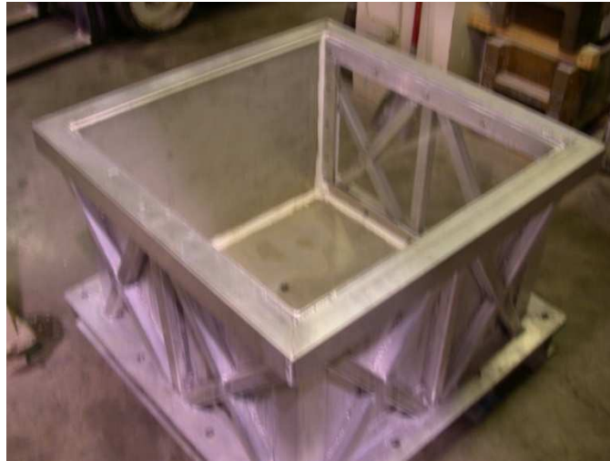
Figure 2-23 – The sample box used for shaking table testing at Ecole Polytechnique - Montreal (Photo by Darcy Joliette).
