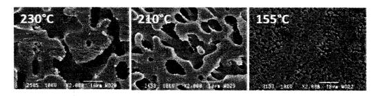
Figure 2.12 Effect of annealing temperature on binary blends morphology (show the pore-size and distribution) (taken from <u>Sarazin and Favis</u>, 2005)
