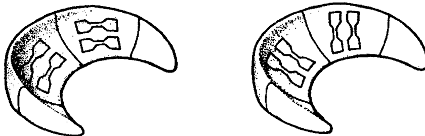
Figure 1. 9 Two dumbbell-shaped tensile specimens were obtained from each slice of tissue, oriented in either the circumferential or the radial direction. Circumferential (left); Radial (right) (Proctor et al., 1989)
