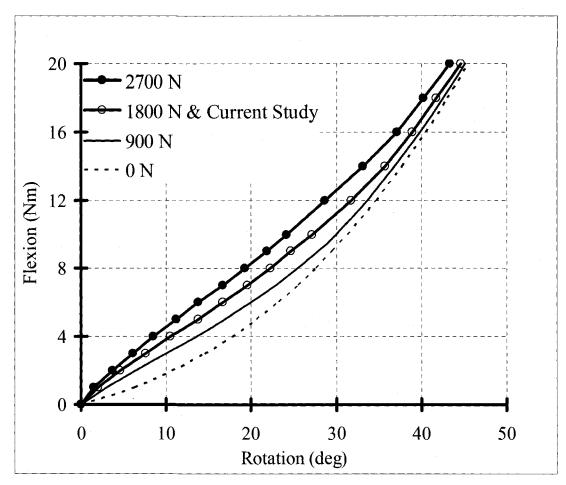
**Figure 6.2** Nonlinear lumbar responses to applied flexion moment under 0, 900, 1800, and 2700 N wrapping compression preloads
