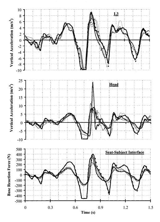
Figure 5.4 Measured and predicted response at L3 (top) and Head (middle) along with reaction force at seat-subject interface (bottom). Three postures considered in experimental studies (i.e. Driving, Bent, and Upright) and two in the current model studies (i.e. Erect, Flexed ) are presented.
