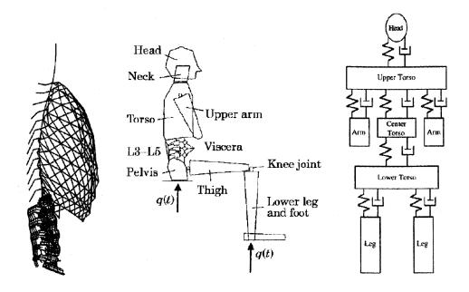
**Figure 1.9** (Left) finite element model (Goel et al 2003), (Middle) an anatomic model (Pankoke et al 1998), (Right) a general lumped parameter model (Goel et al 2001)
