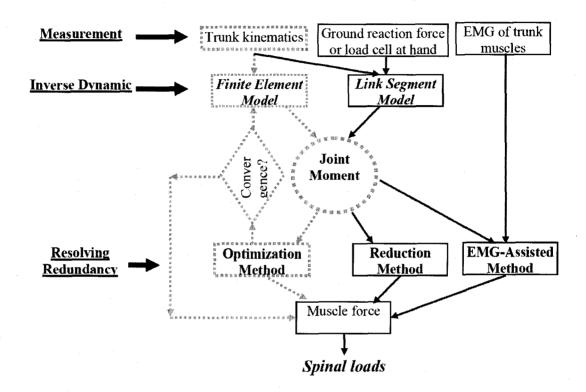
**Figure 1.7** Different modeling approaches for calculation of spinal loads. Both link segment and finite element models use measurement data to calculate joint loads. The 3-D joint moment is, then, partitioned among trunk active-passive components using one (or a combination) of methods for resolving trunk redundancy. Flow of kinematics-based approach is depicted by dashed lines.
