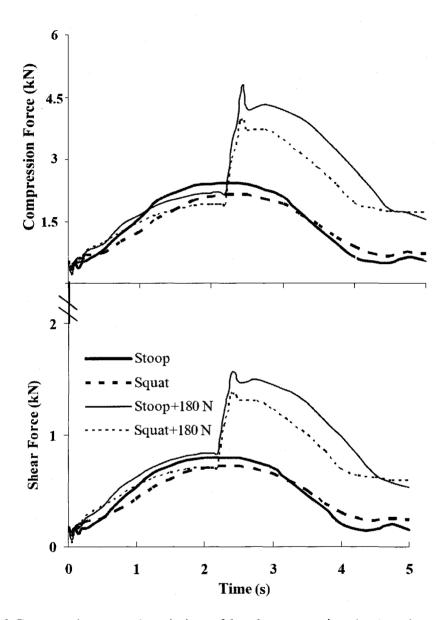
**Figure 2.6** Computed temporal variation of local compression (top) and anterior shear (bottom) forces at the L5-S1 level for different cases. These forces are normal and tangential to the disc mid-height planes.
