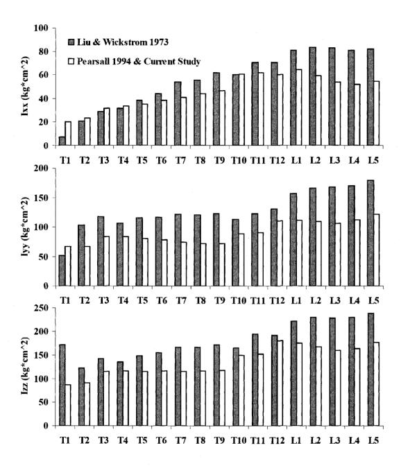
**Figure 6.4** Comparison of trunk segmental mass moments of inertia at different vertebral levels considered in the current study with earlier investigations. x, y, and z represent transverse (lateral), anteroposterior, and longitudinal directions respectively (mass of the T1-L5 section were 22 and 26 kg for subjects considered in Pearsall (1994) and Liu and Wickstrom (1973) respectively)
