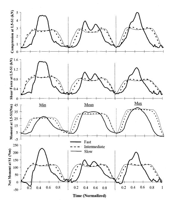
**Figure 4.6** Predicted temporal variation of internal spinal forces at the L5-S1 disc midheight in local directions (compression force, shear force and sagittal moment) and the net moment at the S1 (to be resisted by all muscles and passive ligamentous spine) at the bottom for three subjects 'Min' (left), 'Mean' (middle), and 'Max' (right) at different movement velocities.
