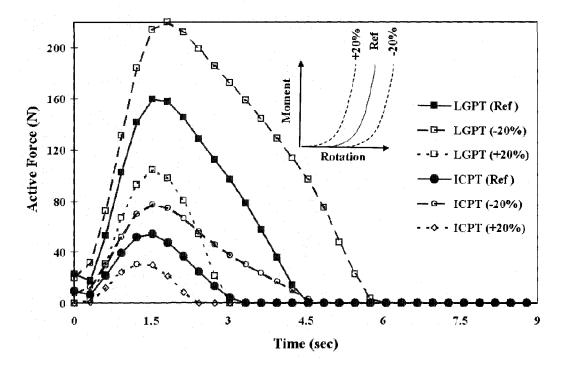
**Figure 6.12** Predicted temporal variation of active force (on each side) in extensor global muscles with time from upright standing posture toward full flexion as the bending stiffness of motion segments is altered by  $\pm 20\%$  at all levels (Arjmand et al., 2008).
