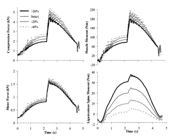
**Figure 3.3** Predicted temporal variation of internal forces at the L5-S1 as well as muscles and ligamentous spine contributions in carrying the net moment at the L5-S1 level for different passive properties in stoop lifting.
