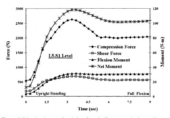
**Figure 6.10** Predicted temporal variation of passive ligamentous loads as well as net external moment at the L5-S1 disc level with time during a slow forward flexion movement (Arjmand et al., 2008).
