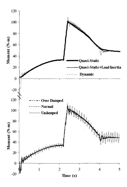
**Figure 2.7** Predicted effect of changes in system dynamics characteristics on the net moment at the T12 level for the squat lift with 180 N in hands; effect of consideration of trunk and load inertias (top) and of damping (bottom).
