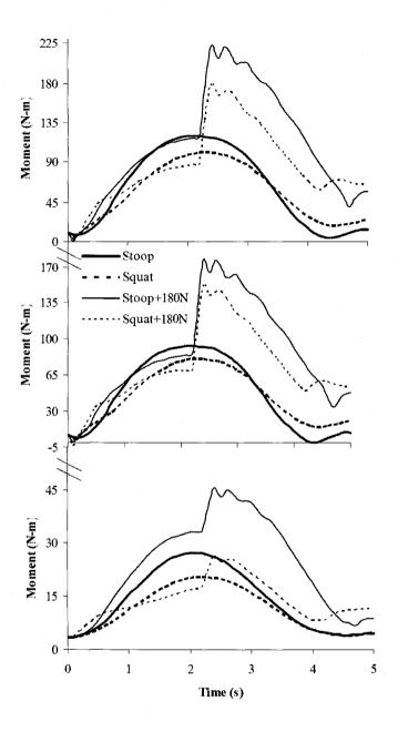
**Figure 2.3** Predicted temporal variation of sagittal moments at the L5-S1 level for different cases (N-m); net external moment (top), portion resisted by muscle forces (middle), and portion resisted by passive ligamentous spine (bottom). For the cases with load in hands, the sharp increase in moments is noted as the load reaches its maximum value of 180 N in 0.2s duration.
