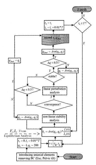
**Figure A.3** Flowchart of the routine written in Python (Python 2.5) to perform iterative stability analyses in Kinematics-based approach at each instance of the time;  $L_i$  denotes the instantaneous muscle length, T denotes total time,  $F_i$  denotes the total muscle force,  $q_i$  is muscle stiffness coefficient, and  $k_i$  is muscle stiffness.
