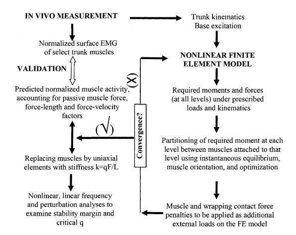
**Figure 5.1** Flowchart for the application of the Kinematics-based approach used to determine trunk muscle forces, internal loads and spine stability under whole body vibration base excitation. Convergence is attained if calculated muscle forces in two successive iterations remain the same.
