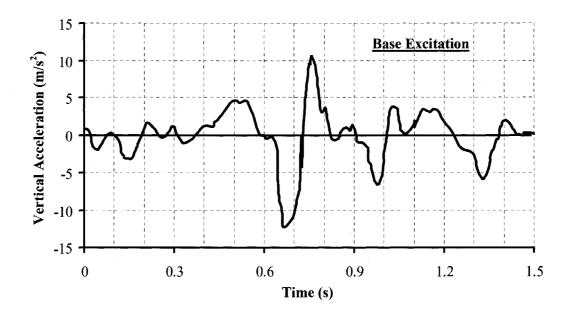
**Figure 5.3** The input random seat vertical acceleration at the base considered in the model based on the measured un-weighted acceleration at the seat-driver interface of a hydraulic excavator (Seidel et al., 1997).
