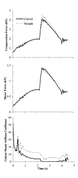
**Figure 3.5** Predicted effect of global muscles simulated either as curved or straight on the L5-S1 compression (top) and anterior shear (middle) forces as well as minimum (critical) muscle stiffness coefficient, q, (bottom) for the squat lift.
