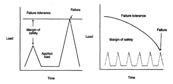
**Figure 1.2** (Left) a margin of safety is observed in the first cycle of sub-failure load. In the second loading cycle, the applied load increases in magnitude, simultaneously decreasing the margin of safety to zero, at which point an injury occurs. (Right) repeated sub-failure loads lead to tissue fatigue, reducing the failure tolerance. (McGill, 2007)
