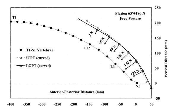
**Figure 6.13** Magnitude and direction of wrapping contact forces on the spine due to wrapping of global muscles (Longissimus Thoracis pars thoracic, LGPT, and Iliocostalis Lumborum pars thoracic, ICPT) for the case with no reduction in lever arms from upright posture under trunk flexion of 65° with 180 N in hands (Arjmand et al., 2006)
