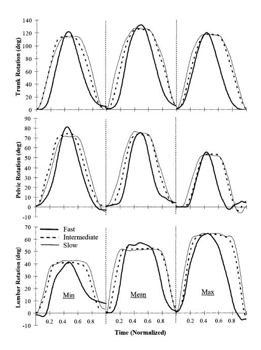
**Figure 4.2** Prescribed thorax (top), pelvis (middle), and lumbar (bottom) rotations in the model for three subjects 'Min' (left), 'Mean' (middle), and 'Max' (right) at three movement velocities based on in vivo measurements. The lumbar rotations are subsequently partitioned in between different levels based on proportions given in the text.
