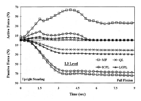
**Figure 6.11** Predicted temporal variation of active force in local trunk extensor muscles (on each side) attached to the L3 level with time during slow forward flexion movement. Muscle forces at other lumbar levels (not shown) follow similar trends (Arjmand et al., 2008).
