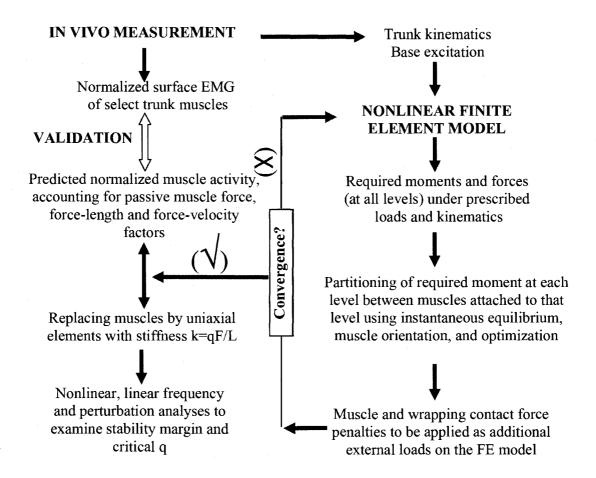
**Figure A.1** Flowchart for the application of the Kinematics-based approach used to determine trunk muscle forces, internal loads and spine stability. Convergence is attained if calculated muscle forces in two successive iterations remain the same.
