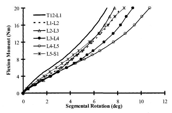
**Figure A.4** Variation of flexion moment with segmental rotation for different lumbar motion segments under 1800 N axial compression.
