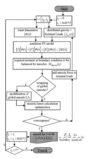
**Figure A.2** Flowchart of the routine written in Python (Python 2.5) to perform iterative equilibrium analyses in Kinematics-based approach at each instance of time;  $L_i$  denotes the instantaneous muscle length, T denotes total time, and  $F_i$  is the total muscle force.
