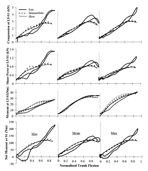
**Figure 6.7** Predicted temporal variation of internal spinal loads at the L5-S1 disc mid-height in local directions (compression force, shear force and sagittal moment) and the net moment at the S1 (to be resisted by all muscles and passive ligamentous spine) for three subjects 'Min' (left), 'Mean' (middle), and 'Max' (right) at different movement velocities. (Results are all normalized with respect to peak trunk flexion of 132°)
