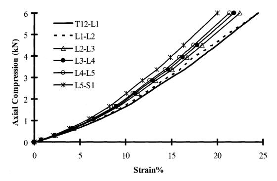
Figure A.5 Load-displacement properties for different lumbar motion segments.
