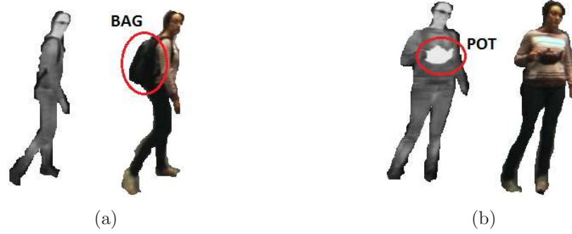
Figure 1.3 Implicit object detection. Human ROIs are extracted using a background subtraction. (a) thermal (left) and visible (right) corresponding human ROIs of a person carrying a bag (b) thermal (left) and visible (right) corresponding human ROIs of a person carrying a hot pot.
