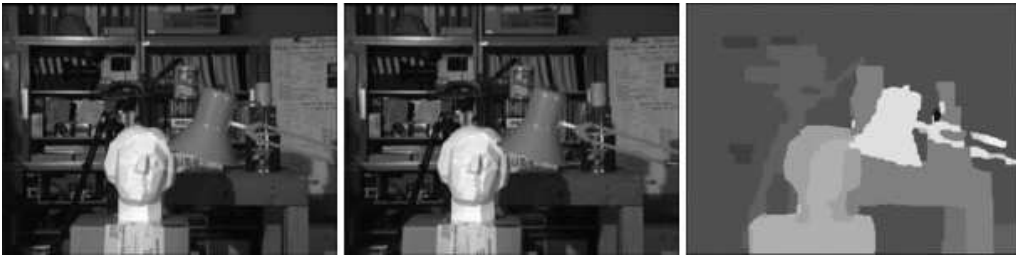
Figure 2.4 Pair of visible images from two view-points (left and middle) and dense disparity map computed using efficient BP (right).
