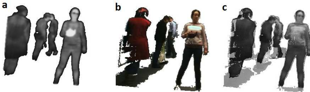
Figure 7.7 Detailed registration a person carrying a hot pot. (a) Foreground thermal image, (b) Foreground background image, and (c) Registration of visible image on thermal image.
