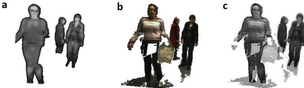
Figure 7.8 Detailed registration of a person carrying a bag. (a) Foreground thermal image, (b) Foreground background image, and (c) Registration of visible image on thermal image.
