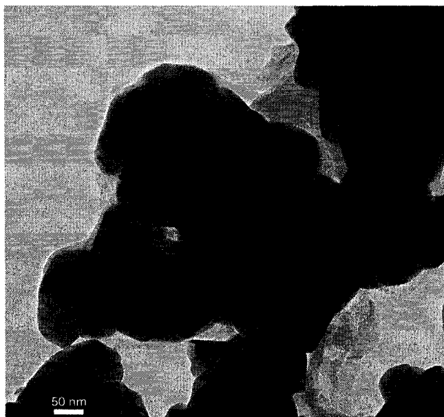
Figure 6.8. TEM image of coated agglomerate of zirconia nanoparticles
