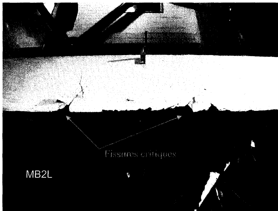
Figure 7.12: MB2L – Fissures critiques
