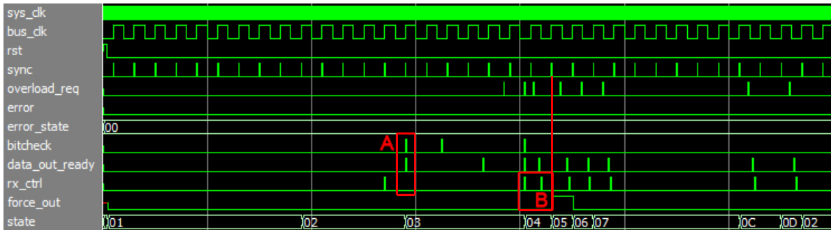
Figure 3.3 Simulation example: FSM reception reception flow
