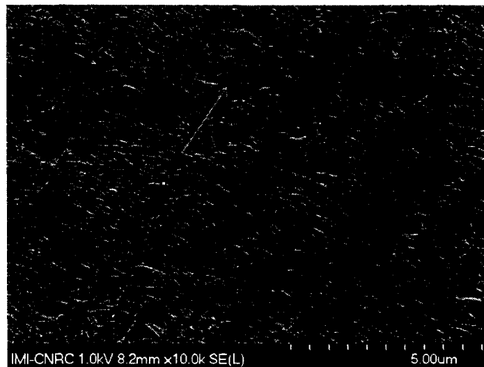
Fig.2.8 A typical row nucleated lamellar structure from HDPE.
